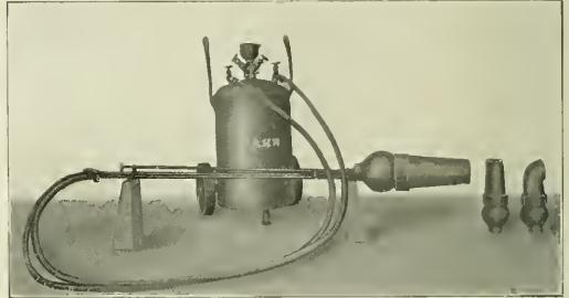
Fig. 1—Mahr Oil Burner for Car Repairs.
